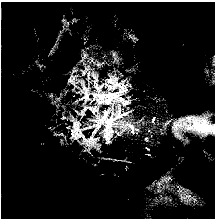
FIG. 1. Vanadium–antimony oxide catalyst, calcined at 820^\circ\text{C} for 24 h in air. Magnification: 1900.
